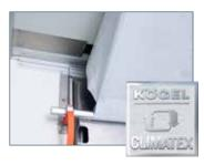
The elongated, wider air duct ensures that the cooling air is guided and distributed throughout the interior even more effectively.
