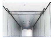
85 millimetre thick sandwich element with insulating core
