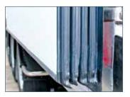
Optimised four-fold lip seal on door to provide secure seal and reduce energy consumption
