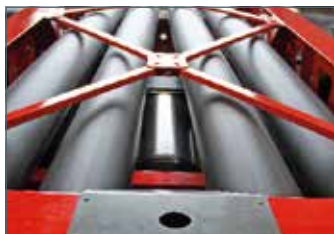
Stowage for hose pipes
