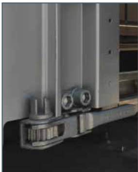
Different equipment for Kögel Mega Ratchet at the front in place of a quick-opening lever
