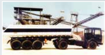
First self-supporting aluminium round-body tipper
