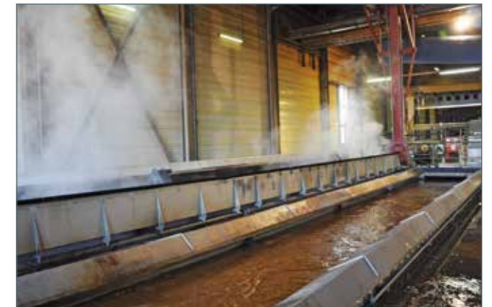
The cathodic dip-paint coating plant is subject to strict testing and inspection procedures.
