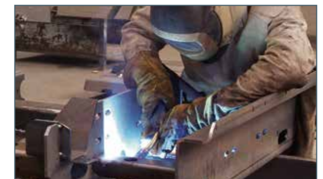
Welding a welded assembly to the frame
