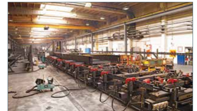
Welding jigs help to achieve extremely precise welding
