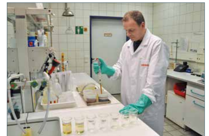
Continuous testing of the stipulated parameters of the baths is carried out in the cathodic dip-paint coating laboratory.
